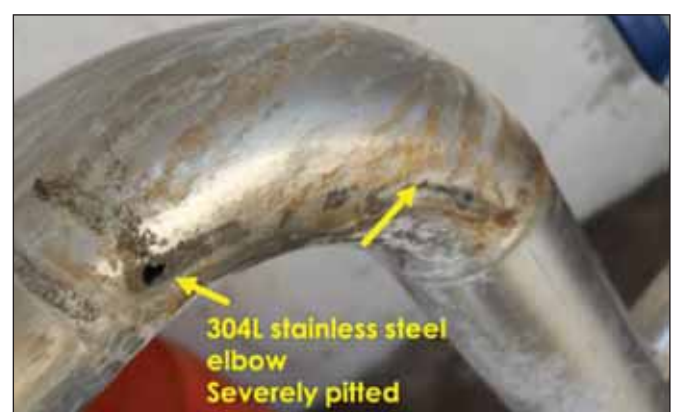
Figure 1: Pitting corrosion of a 304 stainless steel pipe at the weld seam.
