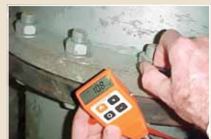
Zinc electroplating coating thickness 10.8µm.
