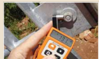
Hot dip galvanized coating thickness on this nut 131µm.
