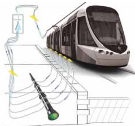
Figure 2: Stray voltage is the occurrence of electrical potential between two objects that ideally should not have any voltage difference between them.
