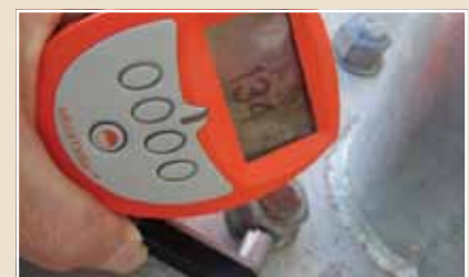
Hot dip galvanized coating thickness on this nut 134µm.
