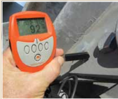
Zinc electroplating coating thickness 9.2µm.
