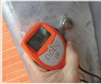
Zinc electroplating coating thickness 11.0µm.
