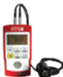
Ultrasonic Wall Thickness
