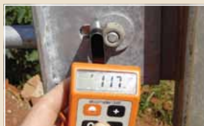
Hot dip galvanized coating thickness on this flat washer 117µm.
