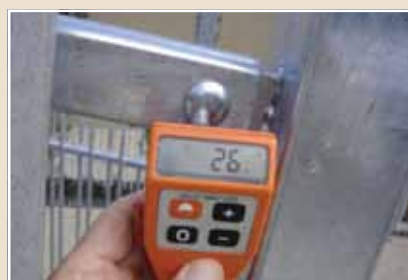
Zinc electroplating coating thickness 26µm.
