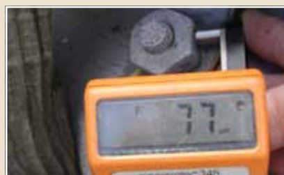
Hot dip galvanized coating thickness on this nut 77µm.
