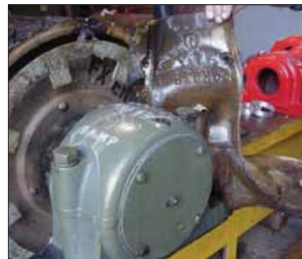
Figure 27: No corrosion on test bearing.
