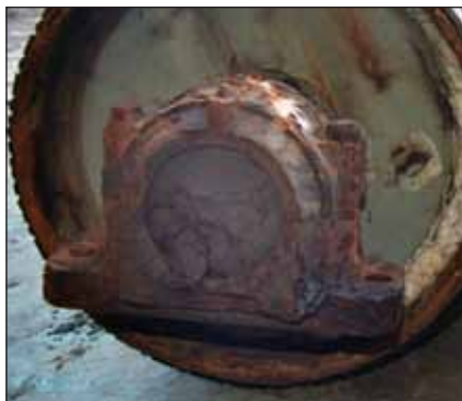
Figure 26: Severe rusting from high salt levels.
