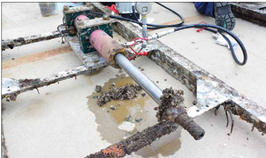
Marine hydraulics using the newly developed HVOF coatings are more resistant to biofouling and are more readily cleaned without damage to the anti-corrosive coating.
