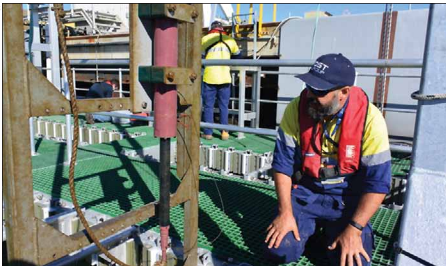
Defence researchers assess the corrosion and anti-biofouling performance of test hydraulic units coated with HVOF coatings at the DST marine exposure site in Melbourne, Australia.
