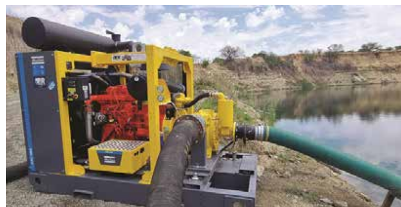
Available from IPR is the Atlas Copco PAC H64 which offers a maximum flow rate of 460m 3 at a maximum head of 150m.
