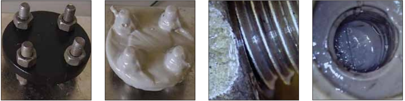
Figure 17: Cyclic test piece before and after coating plus thread and coating interior after test.
