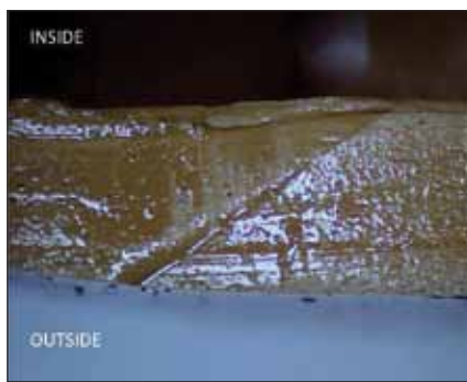
Figure 14: Slight drying on outer edge.
