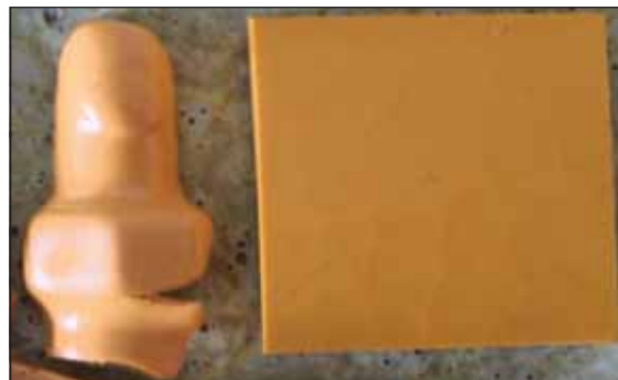
Figure 12: Slight fading after 4 500 hours.
