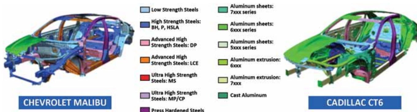
Figure 1. Mixed materials “body in white” for Chevrolet Malibu and Cadillac CT6. Image courtesy of General Motors and from reference 4. Reproduced under a Creative Commons Attribution 4.0 International License.
