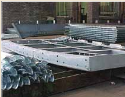
When hot dip galvanizing unsymmetrical components such as this, opposing residual forces can result in distortion.
