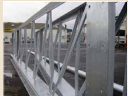
Varying thickness of steel making up a girder can cause differential expansion when dipped into molten zinc. The component may distort after hot dip galvanizing.
