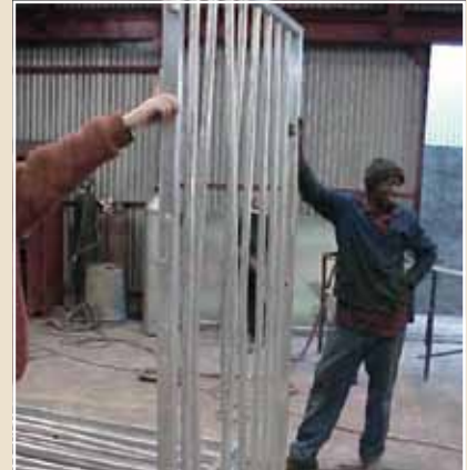
Varying thickness of steel making up a frame can cause differential expansion when dipped into molten zinc.
