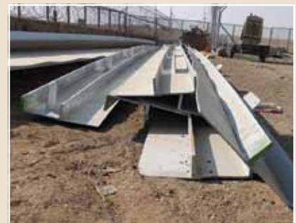
Long thick components welded to long thin plates that are unsymmetrical, can cause distortion of the thinner plate due to different heating cycles in the molten zinc.
