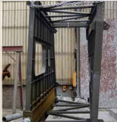
When delivered components are already distorted due to weld imbalances, galvanizers are to notify the client and suggest alternative corrosion control.
