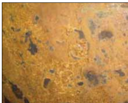
Figure 2: Corrosion on the inside of the produced water tank.
